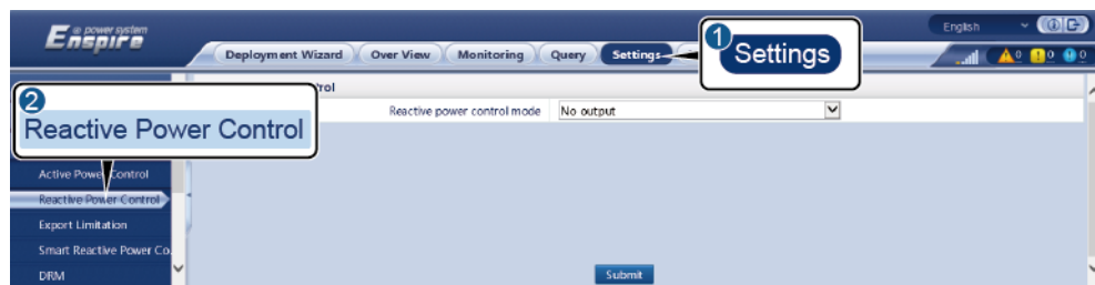
Figure 6-43 Reactive power control
